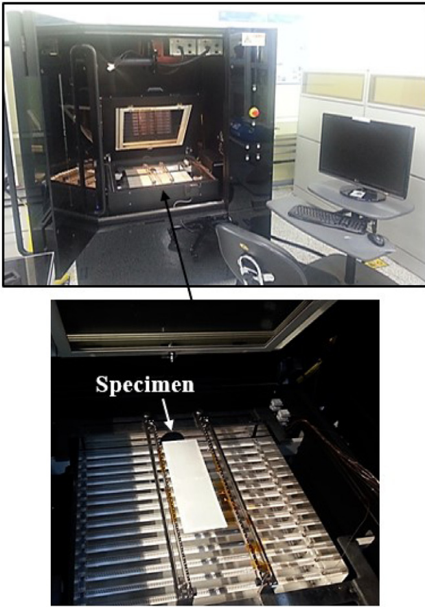
Figure 7. Experimental setup of shadow moiré for PCB warpage measuring.
